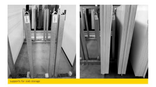
3 mm and 6 mm slabs need at least three support points, distributed evenly along the back of the slab; a full support is recommended - an unused granite or marble slab with sufficient width, for example. The best way to maintain the integrity of the slabs is to keep them in their original packaging or use a full support on the back of the slab such as an unused granite or marble slab which is wide enough.
