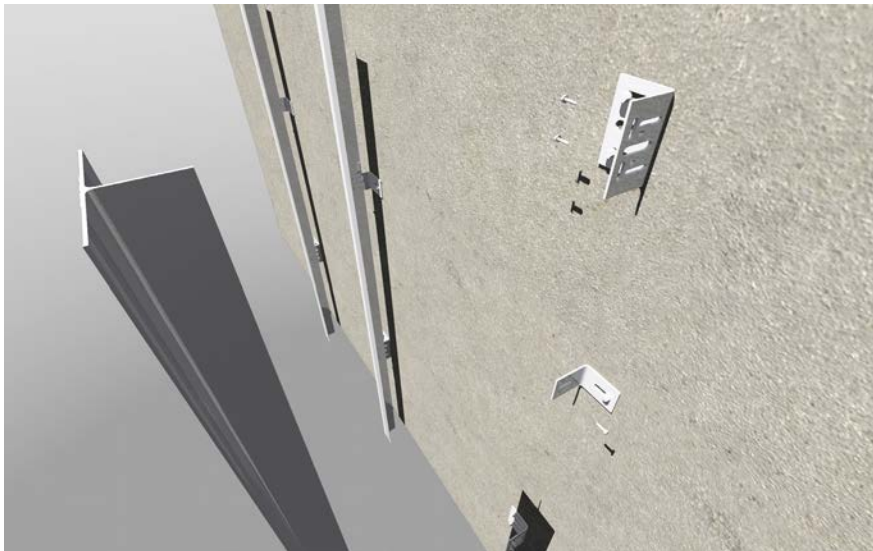
Image 19: HC System installation Step 1
