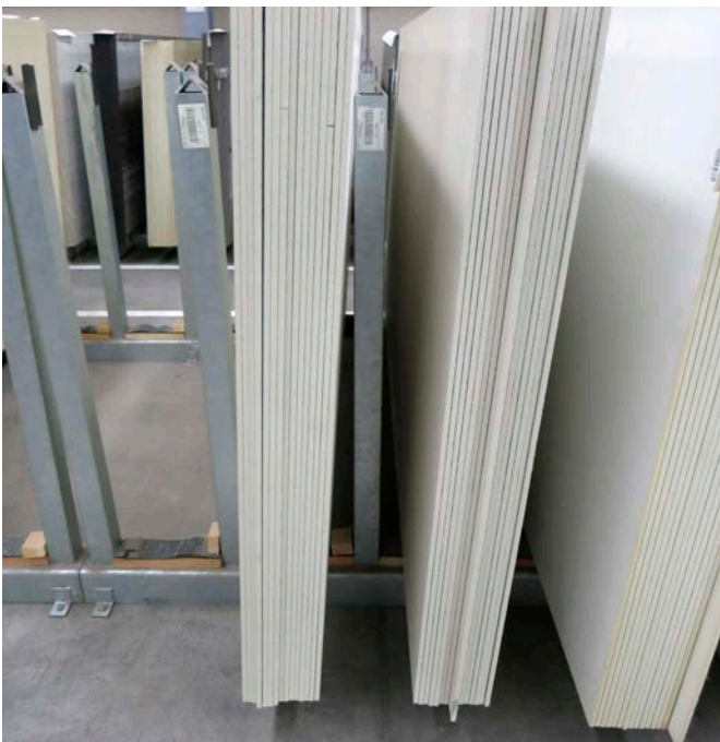
Image 4: 12 mm slabs vertical storage
