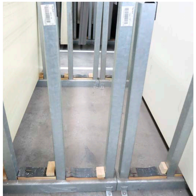
Image 5: Wooden supports beams
