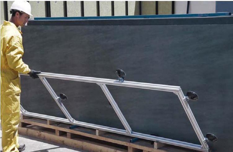
Image 6: Alimunium frame with suction cups
