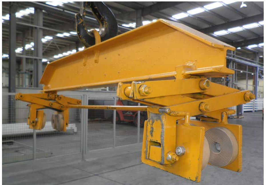
Image 9: Clamp handling for 12 mm slabs
